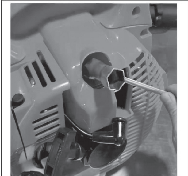
Spark Plug (turn counterclockwise to remove)
