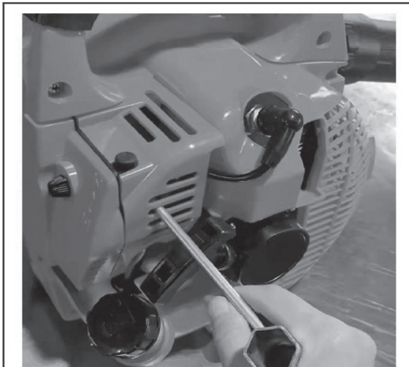
Idle Speed Adjustment Screw(accessible through cowl louver).
